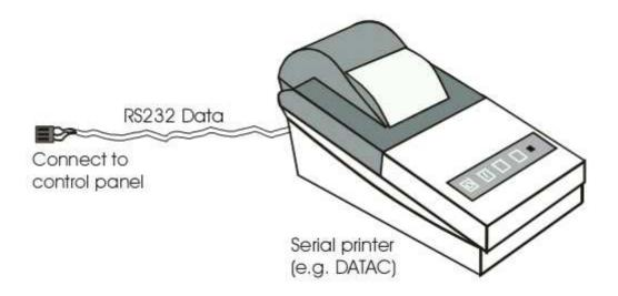
The printer must be set up with the following communication settings: 4800 baud, eight data bits, one stop bit, one start bit, no parity and DTR normal.
