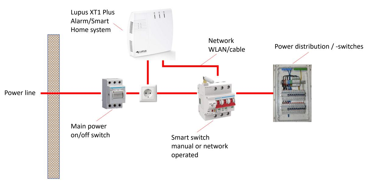
We want to be able to switch the main power supply on and off manually AND using a smart home system.
